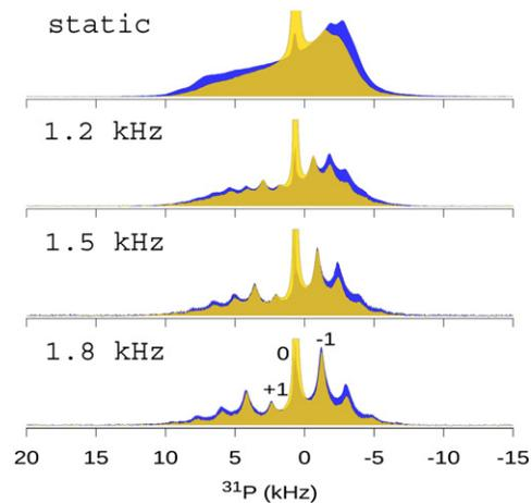
**FIGURE 1** Static and MAS 80 kHz SPINAL-64  $^{31}\text{P}$ -decoupled spectra for 70% DMPE/30% DMPG (blue) and the same lipid system with 2% (mol/mol) maculatin 1.1 added (gold). MAS spectra are scaled to match the  $-1$  spinning sidebands to ease comparison. Opacity is reduced to help discern where spectra overlap.
